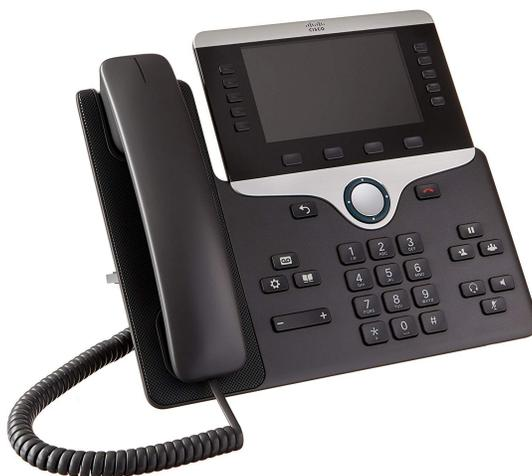
Cisco VoIP devices use CDP for multiple reasons, one of which is PoE (Power over Ethernet) negotiation - The VoIP device can request specific PoE parameters and the switch can enable or disable those parameters and inform the VoIP using CDP. For this reason, CDP is enabled by default in the Cisco VoIP devices, and can not be easily turned off.
