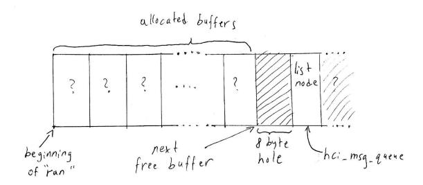
Here, the next 8-byte buffer to be allocated "sits" right before the target 8-byte "list\_node\_t" object. For this layout to occur with a higher probability, it's essential for the target "list\_node\_t" object to "sit" right after the first hole on the "run" that's going to be used for allocation.
