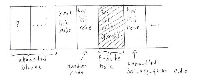
In this scenario, when *bnep\_data\_ind* handles the overflow-inducing datagram that is pointed to by the "handled node", the new *p\_pending\_data* will be allocated in the 8-byte hole. The occurring overflow will than overwrite the unhandled *list\_node\_t*, completing the attack.
